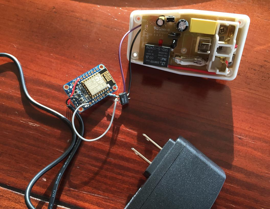
This code uses an Adafruit ESP8266 "HUZZAH" to control 120VAC modules to turn on/off appliances. The program uses the Blynk iPhone Application and Arduino Library. The results are transferred to a cloud server at "Blynk". The Blynk app is downloaded to your phone where the parameters are displayed. In addition, for trending puposes, a graphing
